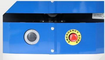
FRED has two buttons on the front and back. The left button tells FRED to move away from you to the next destination on the path. The right button is an emergency stop button.
