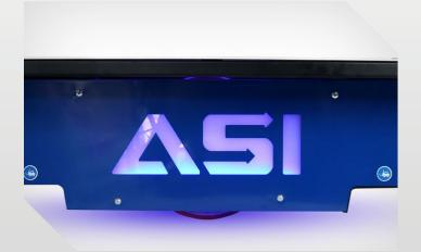
A glowing blue light illuminates the ASI logo on each side of FRED, providing a safety light and a visual battery level indication.
