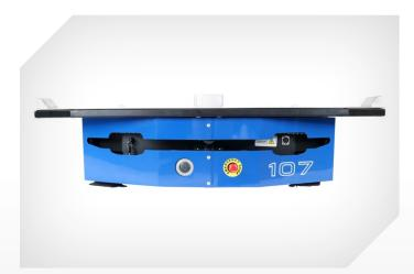
FRED is equipped with safety lasers that detect if an object is in FRED's path. If there is a forklift, pallet, worker, or anything in FRED's way, it stops.
